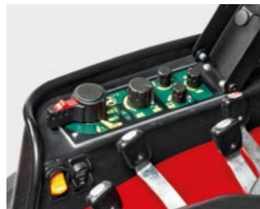
ELECTRONIC LIFTING Electronic lifting at controlled position and effort with damping for road transfer.
