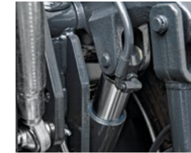
HYDRAULIC SUSPENSION Hydraulic suspension on the UNIFLEX rear powerlift.
