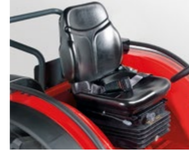
PNEUMATIC SEAT Latest generation with air springs.
