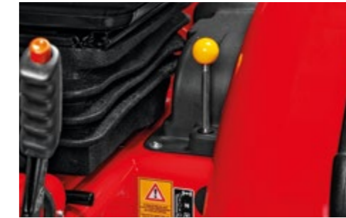
PTO LEVER This command selects the PTO shaft in independent or synchronised mode.
