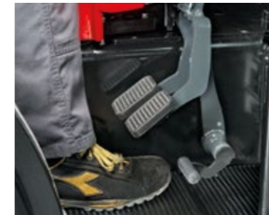
STEERING BRAKES Steering brakes have been introduced to further reduce the turning radius.
