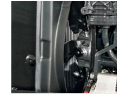
ACS (Air Clean System) Engine cooling fan with air flow reversal. Reduces the need for cleaning the front grille, ensuring more constant engine cooling.
