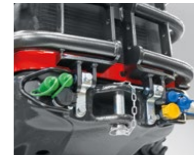
FRONT QUICK RELEASE COUPLINGS Front powerlift > 6 couplings replicated on the rear, of which 2 with double effect + 1 electronically adjustable continual delivery and 1 simple effect.
