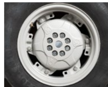
CAST IRON REAR WHEEL FLANGES With six attachment points, to balance the tractor.
