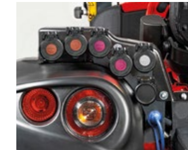
HYDRAULIC SYSTEM Electro-proportional hydraulic system controlled by joystick with double driver safety system and integrated control unit with user-adjustable settings - 12 rear quick couplings. External lifting control.
