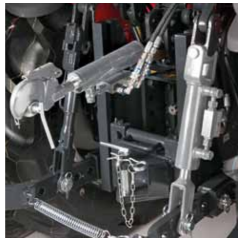
Joystick-controlled* vertical hydraulic tie-rod for practical adjustments from the driving position.
