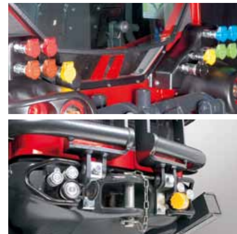
11 rear quick-couplers, 6 of which replicated at the front (opt).
