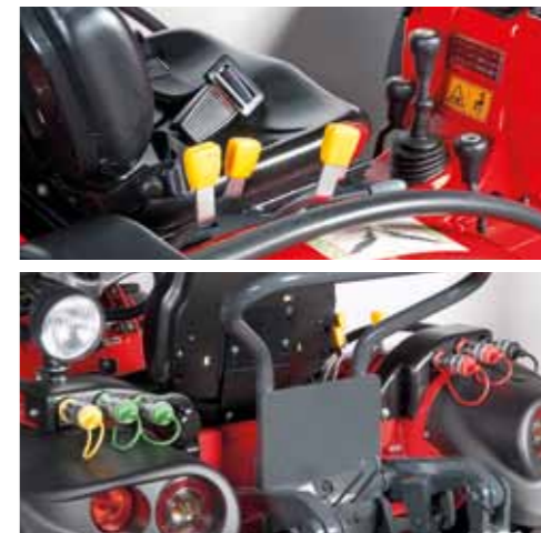
Hydraulic system with 4 double-acting manifolds, 1 single-acting, 1 continuous flow manifold + oil return tap.
