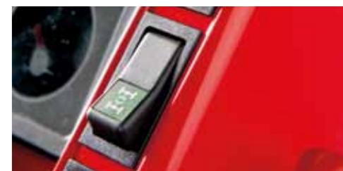
The rear differential lock prevents slipping and optimizes traction. The front traction disengagement is useful when travelling along roads and prevents damage from being done to delicate grounds.
