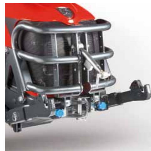
The front lift* optimizes work combined with rear tools.
