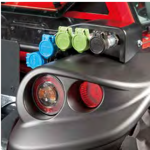
Hydraulic system with 1 double-acting manifold, 1 double-acting with floating position + 1 oil return tap. Total: 5 rear connectors.
