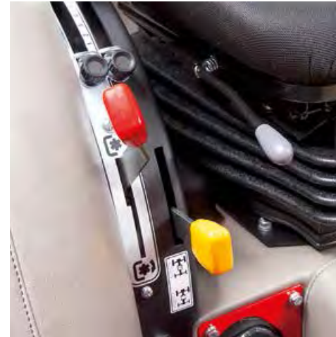
Two speed PTO: 540 rpm, 540 E (750 rpm) and synchronized with gear speeds.
