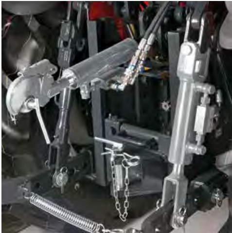
Vertical hydraulic tie-rod and 3-point hitch* allow adjustments to be made from the driver's seat (for the model 10900).
