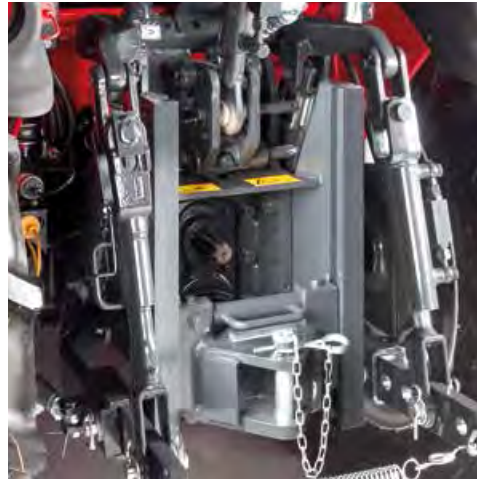
The slider* tow hook with rapid vertical adjustment, is used to optimize the connection height of the towed equipment.
