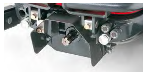
The front PTO* (only for the model 7800) 1000 rpm with electro-hydraulic controls and progressive engagement with safety button is maintenance free.
