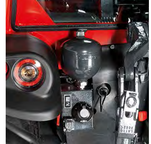
Hydropneumatic suspension with automatic pressure control.
