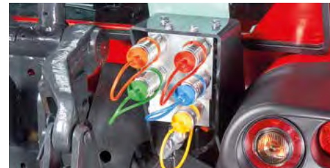
Hydraulic system with electro-hydraulic control with joystick: 2 double-acting manifolds, 1 single-acting, 1 oil return tap. Total: 6 rear quick-couplers.
