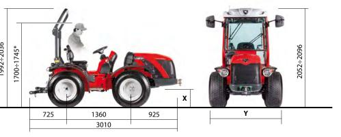
\*Height calculated with the operator of average height sitting (mm 1750)
