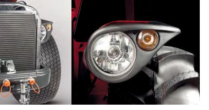
The solid **cast-iron bumpers** protect the engine and radiator and increase the stability of the vehicle thanks to the greater weight on the front axle.
